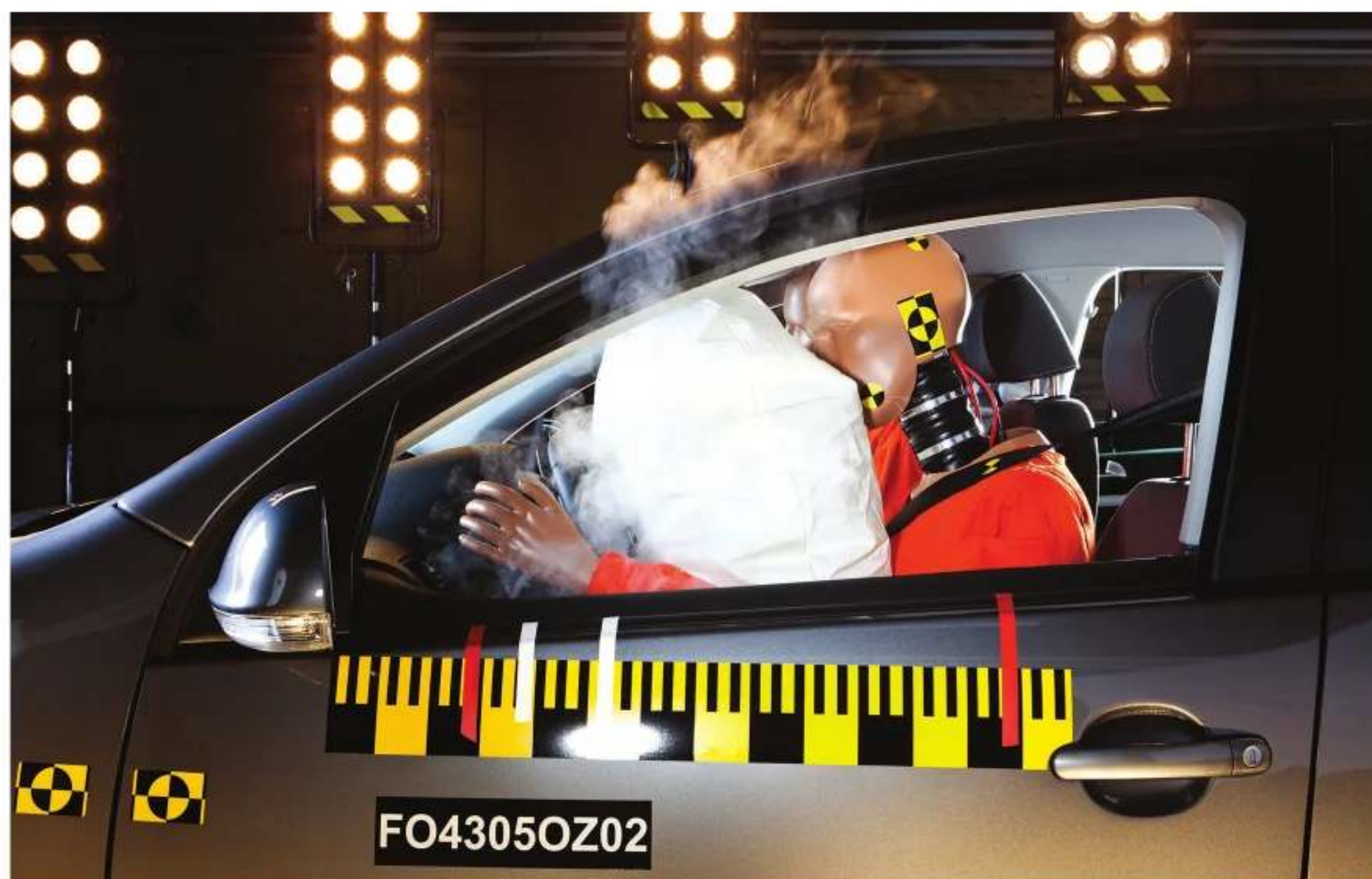
Figure 11 The decomposition of sodium azide, which produces a gas, is the chemical reaction that inflates air bags.
