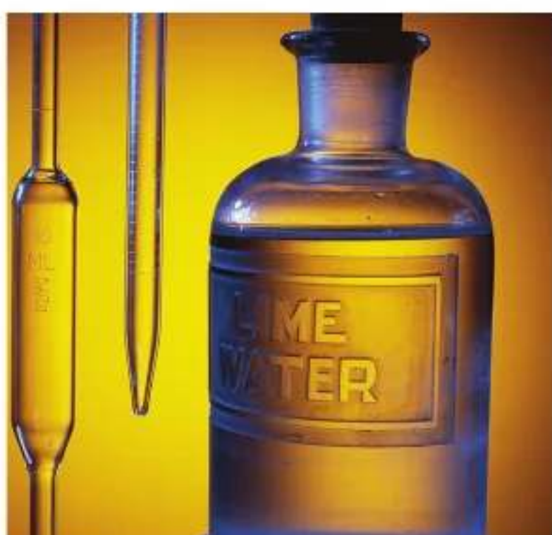
Figure 6 The frosted-looking portions of this glass were chemically etched using hydrogen fluoride (HF), a weak acid. Hydrogen fluoride reacts with silica, the major component of glass, and forms gaseous silicon tetrafluoride (SiF 4 ) and water.
