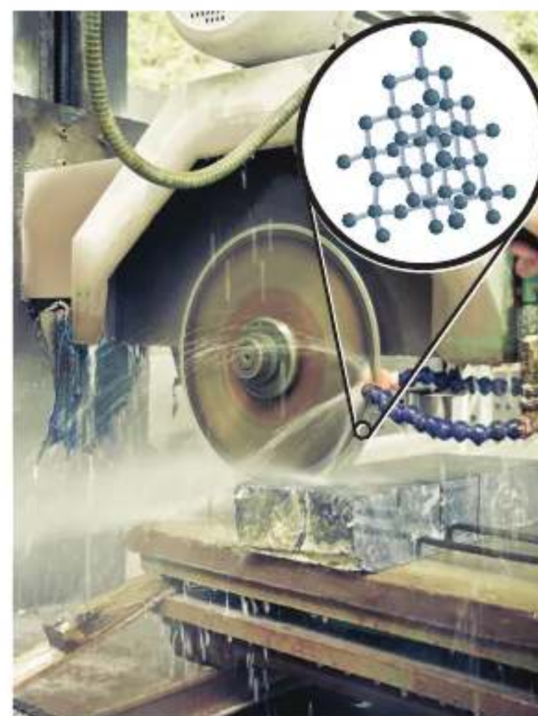
Figure 27 Network solids are often used in cutting tools because of their extreme hardness. Here, a diamond-tipped saw blade cuts through stone.
