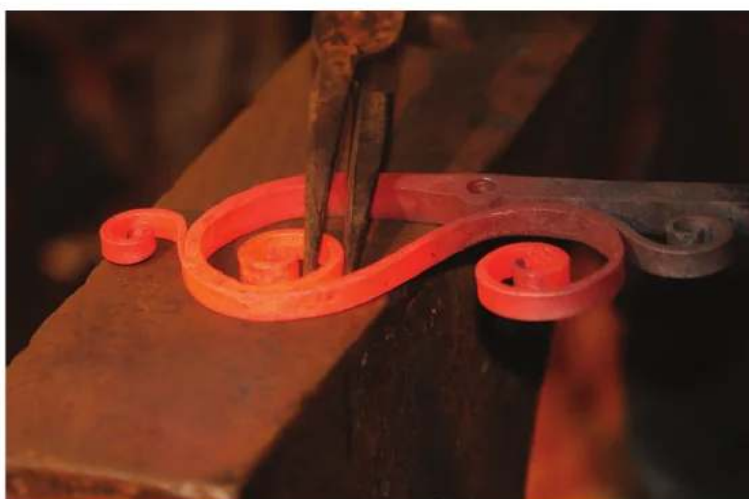
Figure 6 The wavelength of the light emitted by heated metal, such as the iron above, depends on the temperature. At room temperature, iron is gray. When heated, it first turns red, then glowing orange.
