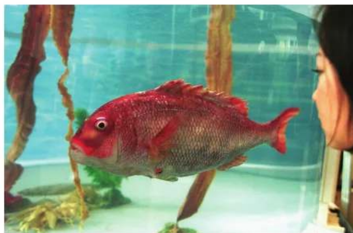
Figure 7 Scientists developing submarine technology created this robot that looks and swims like a real fish. Its body is made of a silicon resin that softens in water.
