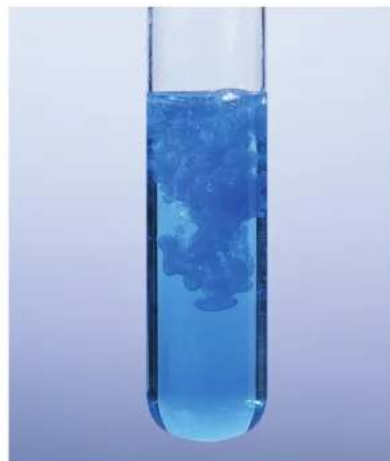
Figure 15 When aqueous sodium hydroxide is added to a solution of copper(II) chloride, the anions ( OH^- and Cl^- ) change places. The resulting products are sodium chloride, which remains in solution, and copper(II) hydroxide, the blue solid in the test tube.
