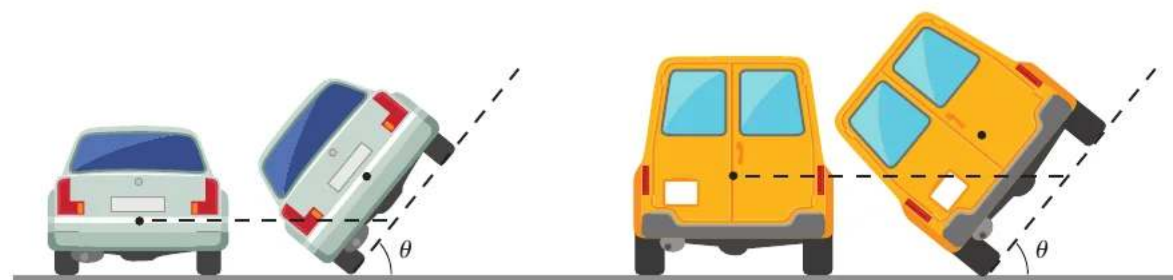
Figure 19 Larger vehicles have a higher center of mass than smaller ones. The higher the center of mass, the smaller the tilt needed to cause the vehicle's center of mass to move outside its base and cause the vehicle to roll over.
