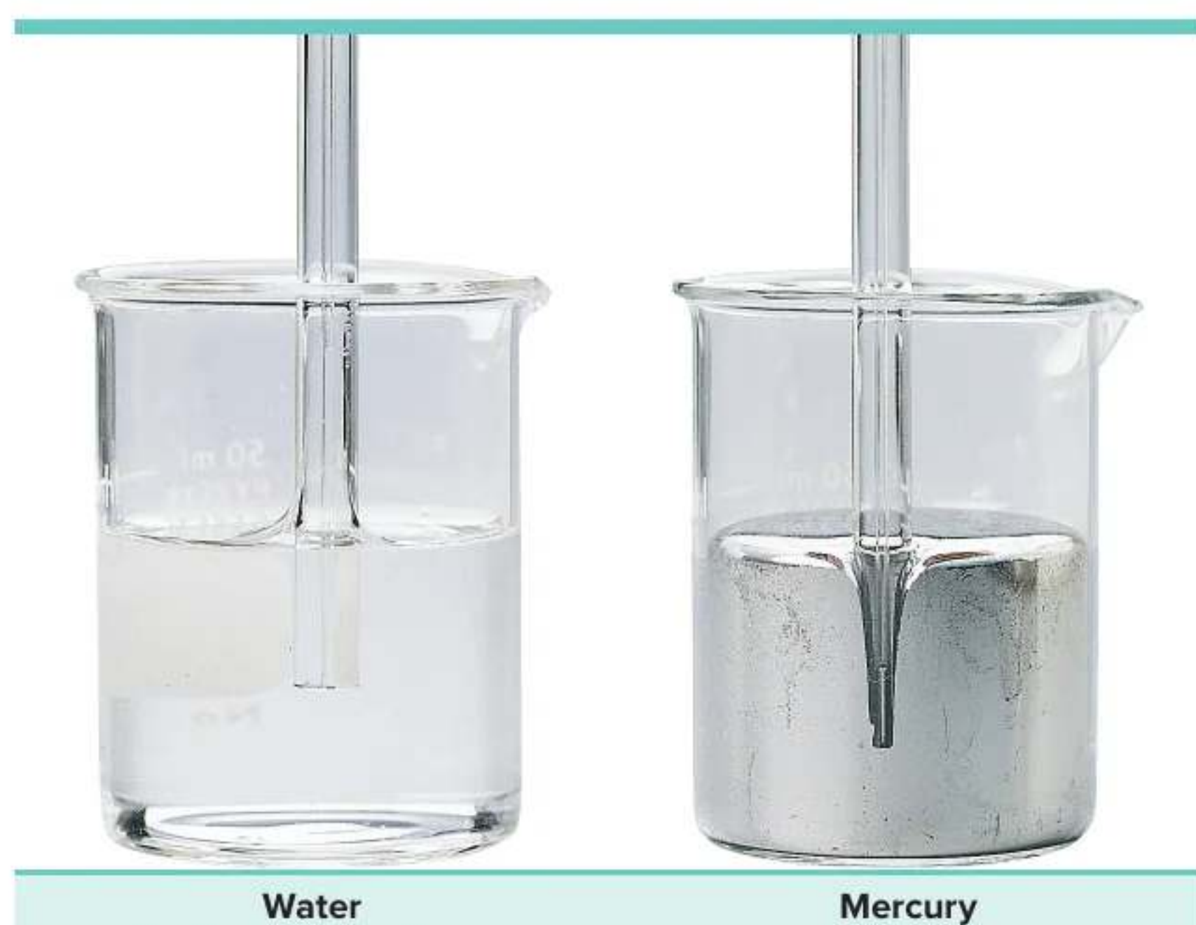
Figure 8 Due to adhesive forces, water climbs the outside wall of the glass tube. In the mercury, however, the forces of attraction between mercury atoms are stronger than any adhesive forces between the mercury and the glass. Therefore, the mercury is depressed by the tube.
