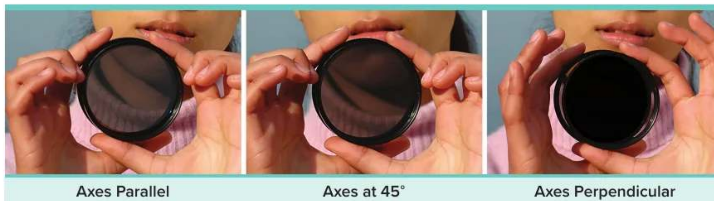
Figure 20 Polarizing filters with their axes parallel will allow the light with the same orientation to pass. With the polarizing axes at a 45^\circ angle, the filters allow some light to pass. If the axes of the filters are perpendicular, the second filter will block the light that has passed through the first filter.
