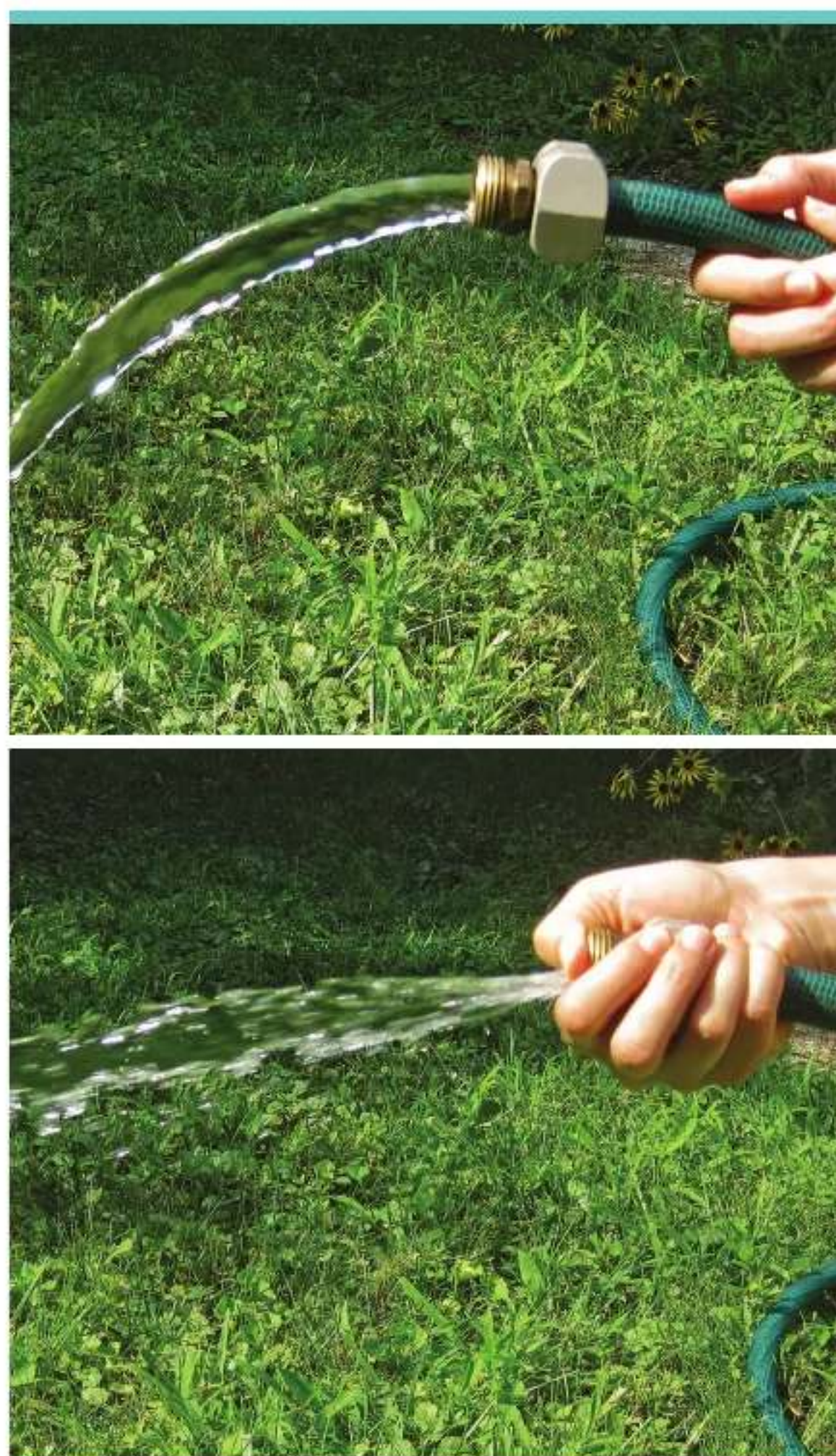
Figure 14 You can demonstrate Bernoulli's principle by narrowing the opening of the hose as water flows out. As the velocity of the water increases, the pressure it exerts decreases.
