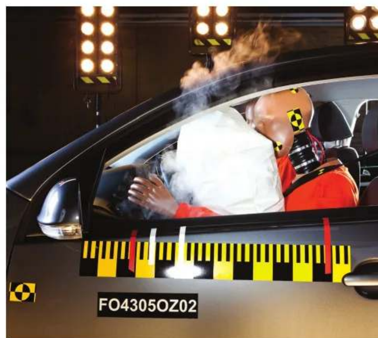
Figure 3 An air bag reduces injuries by making the force on a passenger less and by spreading that force over a larger area.
