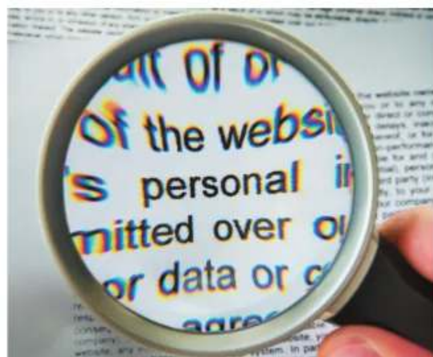
Figure 33 Simple lenses, such as the one shown in the photo on the left, exhibit a rainbow fringing effect called chromatic aberration. Achromatic lenses reduce chromatic aberration.
