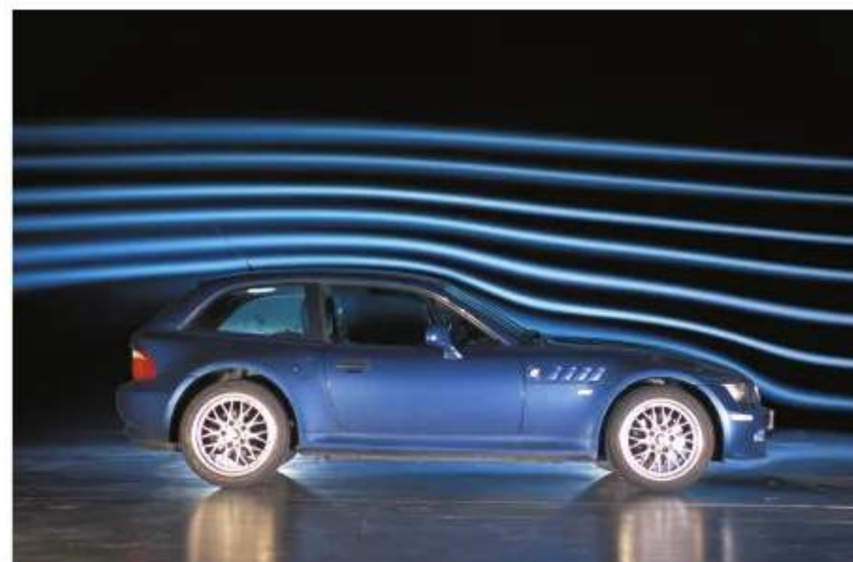
Figure 17 The streamlines show the air flowing above a car in a wind tunnel.
